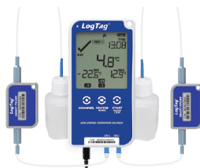
LogTag UTRED30-16 CP Kit with Dual Smart Probe
